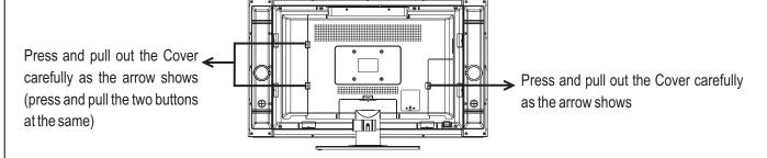
Before you connect external devices with the unit, please removing the Back Cover. After finishing connecting, aim the insertion tabs toward the locating groove, then carefully push the Cover until the Cover locks in place with a click.
